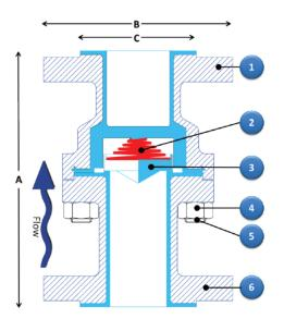
The FPCV embodies all of the features of the WPCV, but has the additional benefit of providing the valve within bolted flange ends, making installation simple and fitting in standard valve face to face spaces.
