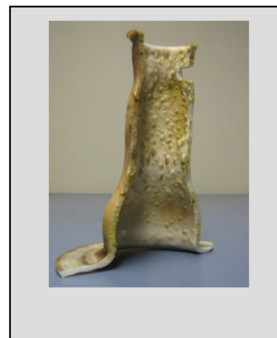
Typical permeation failure of isostatically formed liner
