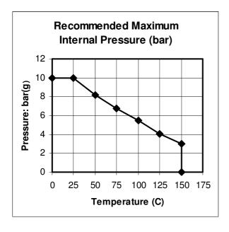
However, in one case, the flanges are the limiting factor. This is for BS10 Table D flanged LGSGs. Here the pressure is limited to a maximum of 6.9 barg at the low temperature end of the range, and by the graph for higher temperatures.
